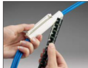
Insert end of tool into the end of Split Harness Wrap. Begin pulling the tool making certain that the Split Harness Wrap is feeding over the wire bundle.
