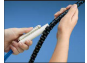
Hold end of Split Harness Wrap and wire bundle while continuing to pull the tool, inserting the wire bundle into the length of the Split Harness Wrap.
